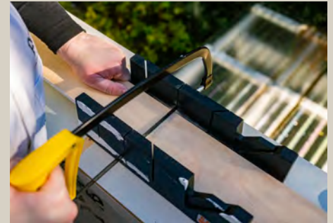
Above: Carefully cut your door panels to the desired lengths for your door. You can have these cut to size at your local timber supplier if you prefer.
